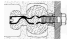
Figure 8.11 Resin fixing with net sleeve
