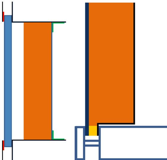
Figure 1 – Shadow box (left), glazed spandrel (right)
