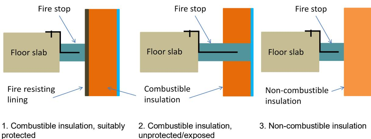
**Figure B1 – Fire stopping details – spandrel zones**
